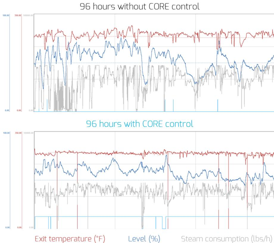
*Top: Cooker - Discharge temperature without CORE control.*
